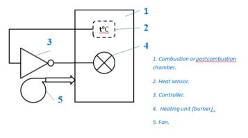
Fig.1. Incinerator control scheme
