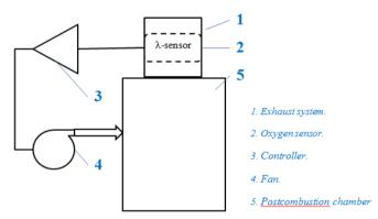
Fig.3. Scheme of control of efficiency of combustion according to oxygen
