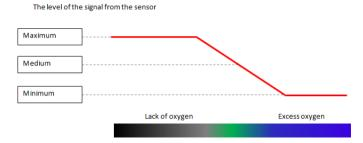
Fig.2. Diagram of operation of the oxygen sensor. Levels of the signal.
