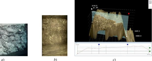
Fig. 1. The fracture surface of the sample: a – the optical macrostructure x40; b - macrostructure in Optimal Image mode; c – 3D structure with profilograms on the highlighted section
