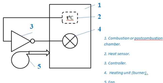
Fig.1. Incinerator control scheme
